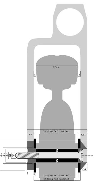
Notes 5.5mm Ø bolt 6.0mm Ø hole 12.0mm Ø pipe bearing
