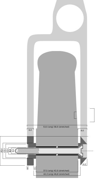
Notes 5.5mm Ø bolt 6.0mm Ø hole 8.0mm Ø pipe bearing
